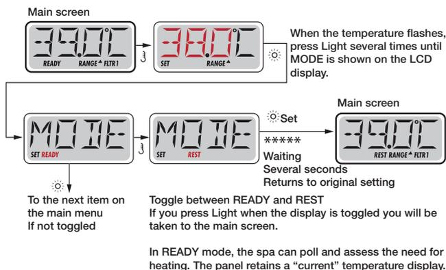
REST mode does not poll, and heating runs only during filter cycles. The panel does not always display the current temperature.
